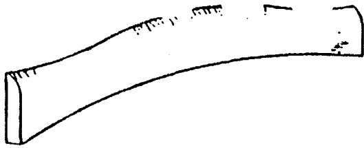
Type of jlg required for shaping and moulding curved chair backs, etc.
